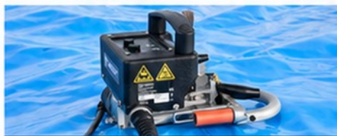
Thin membrane welding
